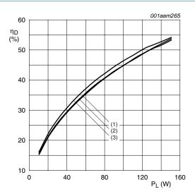
$V_{DS} = 50 \text{ V}; I_{Dq} = 50 \text{ mA}; t_p = 300 \text{ } \mu\text{s}; \delta = 10 \text{ } \%.$
