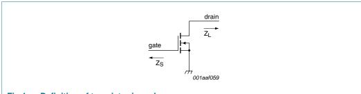
Fig 1. Definition of transistor impedance
