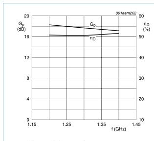
$V_{DS}$  = 50 V;  $I_{Dq}$  = 50 mA;  $t_p$  = 300  $\mu s; \, \delta$  = 10 %.
