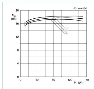
$V_{DS}$  = 50 V;  $I_{Dq}$  = 50 mA;  $t_p$  = 300  $\mu s; \, \delta$  = 10 %.
